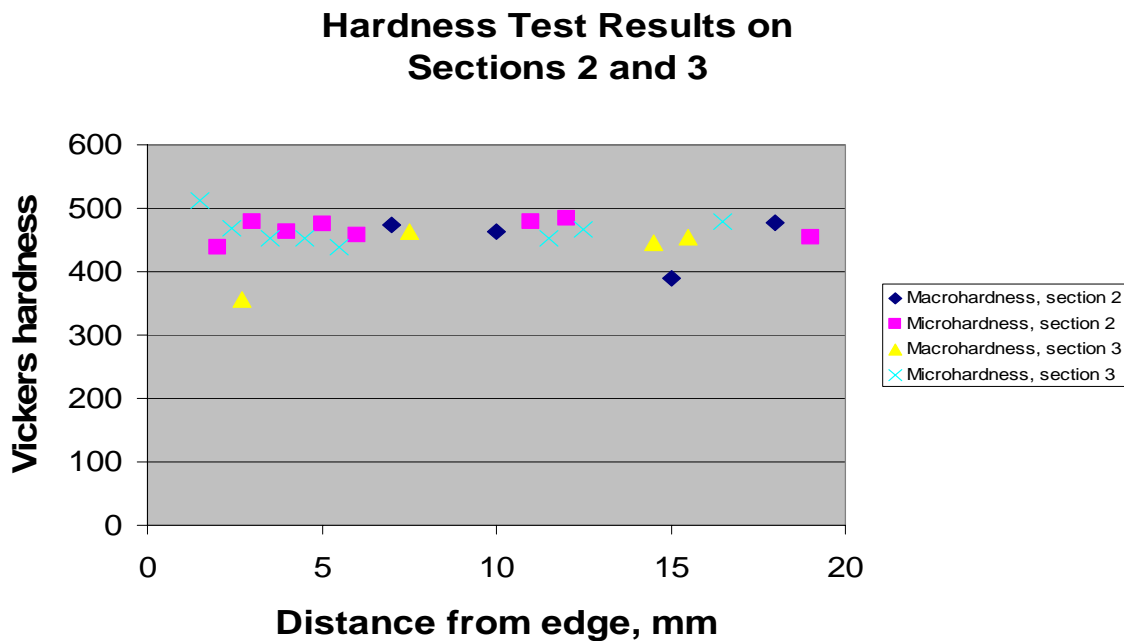
Figures 4. Test results from sample #1. The graph gives the results from the two samples taken away from the heel. (See figure 2 for the position of these samples.) There is little change in hardness at these positions as the blade edge is approached.
